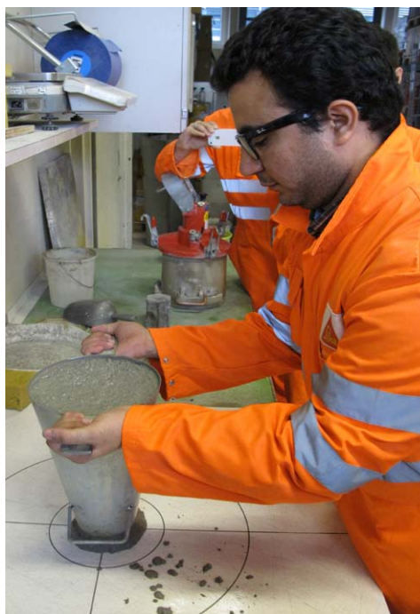
Preparing self-compacting concrete
